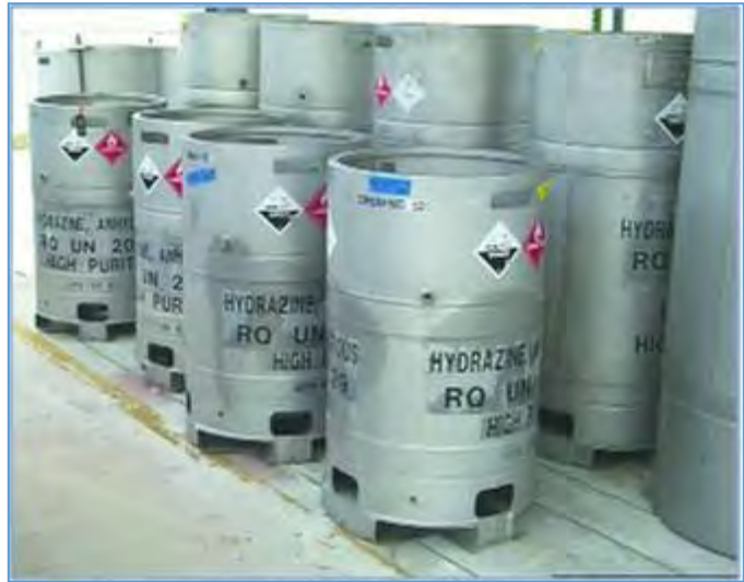
Imagen 57: contenedores de 34 galones de hidrazina anhidra de acero inoxidable serie 300. (MTCR Equipment, Software and Technology Annex Handbook, Third Edition (May 2005))
